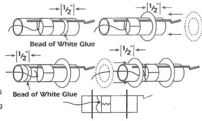
A. Apply white glue around inside edge of Yellow Motor Mount Tube as shown.
